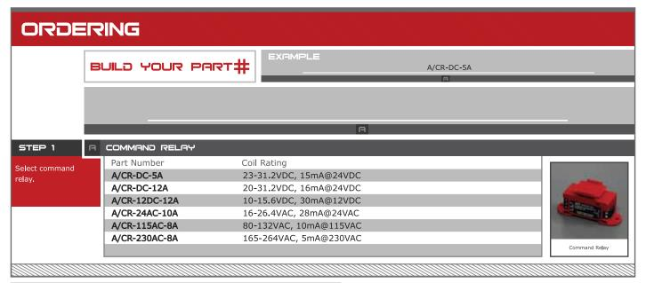
All Current Sensors, Switches and Command Relays have a UL94-5VB flammability rating for the enclosure.
